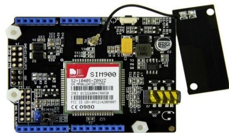
Fig. 3. GPRS SIM900 Arduino Shield
