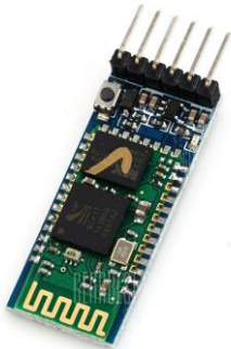
Fig. 4. HC05 Bluetooth radio
